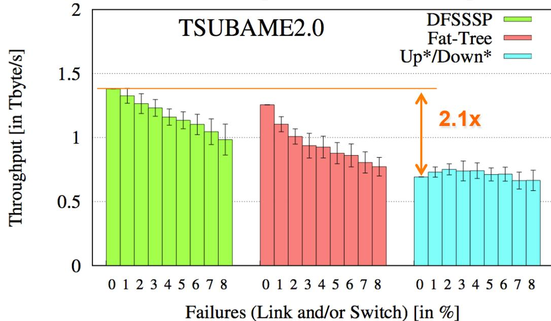
Switch and link failures (1 : 13 ratio)
