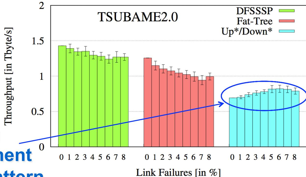
Link failures only (1% annual failure rate)
